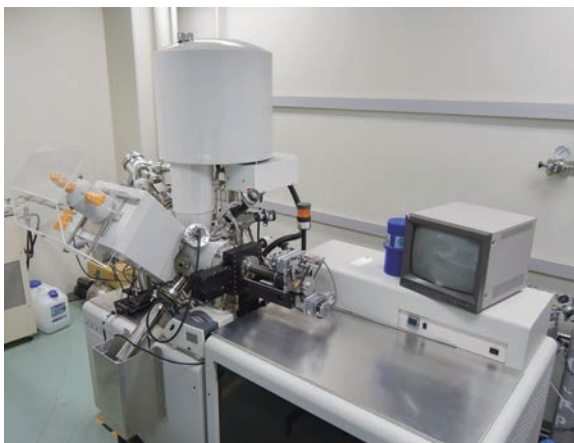
X-ray photoelectron spectroscopy system (ESCA)
