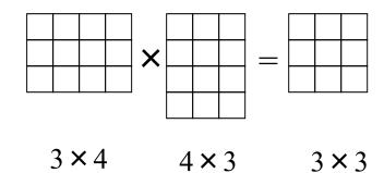
**Example:**  $A_1$ =10 × 20 matrix,  $A_2$ =20 × 5 matrix,  $A_3$ =5 × 25 matrix.  $((A_1 \times A_2) \times A_3)$  require  $(10 \times 20 \times 5)+(10 \times 5 \times 25)=2250$  ops.  $(A_1 \times (A_2 \times A_3))$  requires  $(10 \times 20 \times 25)+(20 \times 5 \times 25)=7500$  ops. Thus, the former needs less operations.
